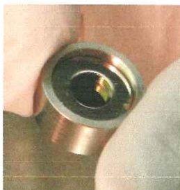
FIG 2: Output Face open end magnet and Faraday rotator.
