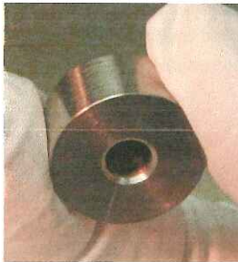
FIG 1: Isolator IO-5-1550-AP1 Input Face polarizer axis parallel to scribe line
