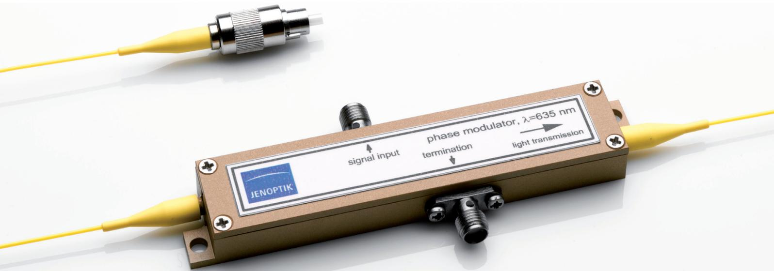
The Integrated Optical Phase Modulator is a compact fiber-coupled electro-optical modulator that works based on  $\text{MgO}:\text{LiNbO}_3$  and  $\text{LiNbO}_3$  crystals. Providing fast electro-optical response, it allows phase modulation with frequencies as high as the Gigahertz range. Available modulators can handle wavelengths in the visible and the infrared spectral range.
