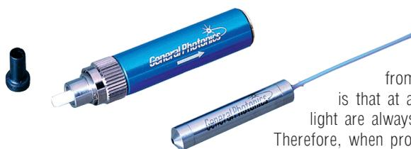
The Faraday rotator mirror is a fiber optic polarization rotation mirror designed for fiber optic networks and measurement applications. The state of polarization (SOP) of the reflected light is rotated 90 degrees
