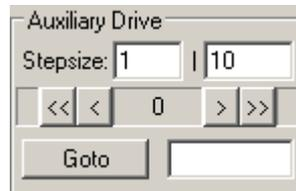
Pressing the arrow buttons moves the motor in the respective direction. The < and > buttons move the motor by the number of steps entered in the left *Stepsize* field, the << and >> buttons by the number of steps entered in the right *Stepsize* field. By pressing the *Goto* button, the motor moves to the absolute position entered in the field next to the button.
