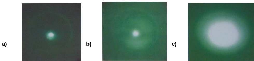
Figure 20: a) IR image of the cladding mode, a bright sharp dot inside a ring. b) IR image of the out coupling mode, core and cladding mode are mixed. c) IR image of the core mode.
