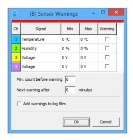
Generate warnings when a sensor falls below or exceeds a minimum or maximum value.
