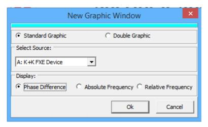
You can display data from just one source (Standard Graphic, scale labels left) or from two sources (Double Graphic, scale labels left and right). FXE devices can choose between different forms of presentation (e.g., phase or frequency).
