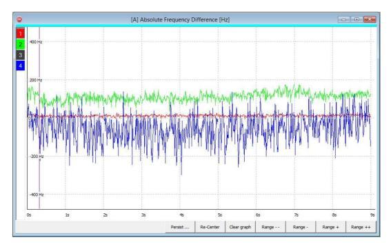
If a graphic window is selected, further operating options are displayed as buttons at the bottom of the window. These are:
