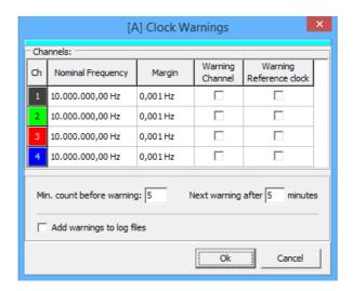
Generate warnings when the measured frequencies or the reference clock leave a predetermined range. Since a reference clock deviation can't be measured directly, at least 2 input frequencies are monitored. If these show deviations at the same time, a reference clock warning is generated.
