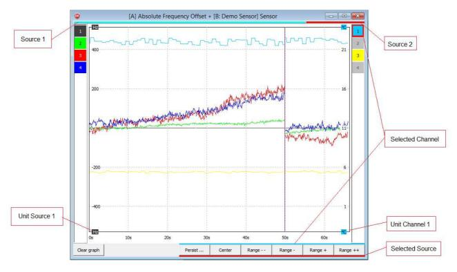
For the second source, the channel selection and scaling of this source is also shown on the right. Since there are devices that can provide different measures (such as temperature and humidity sensors), the scaling for each channel can also be set separately.
