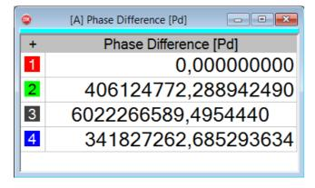
By clicking on the + symbol, a dialogue is opened enabling the selection of displayed channels and the use of several columns, e.g. for the parallel representation of frequency and phase in a window.
