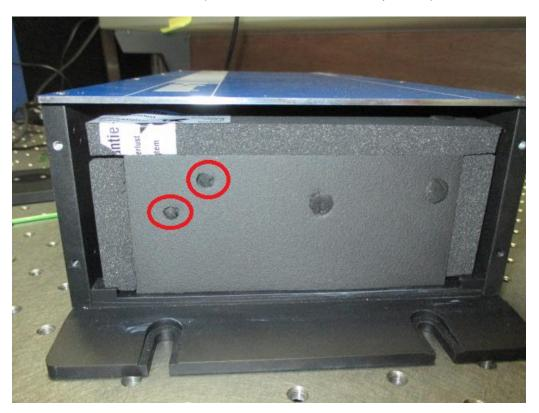
4) Now you have access to the mounting screws for the mirror mount inside the cavity. To adjust the mirror, use a metric 1, 5 mm hex-wrench and slide it carefully in one of the two holes (see below picture). The upper right hole pivots the mirror around the horizontal axis, the lower left hole around the vertical axis. There is some wiggling room when you slide the wrench in the hole.
