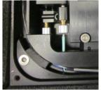
Carefully try to optimize the mirror alignment. Only very tiny adjustments are probably required. The higher the measured monitor power (or DC value) the better. The main problem of this adjustment is that you don't have a real "reading" of the screw positions, so it is difficult to come back to the initial position. If you have reached the maximum DC value/optical output power - ideally close to the DC value reported in your test report, you can now try to find a mode lock state.
