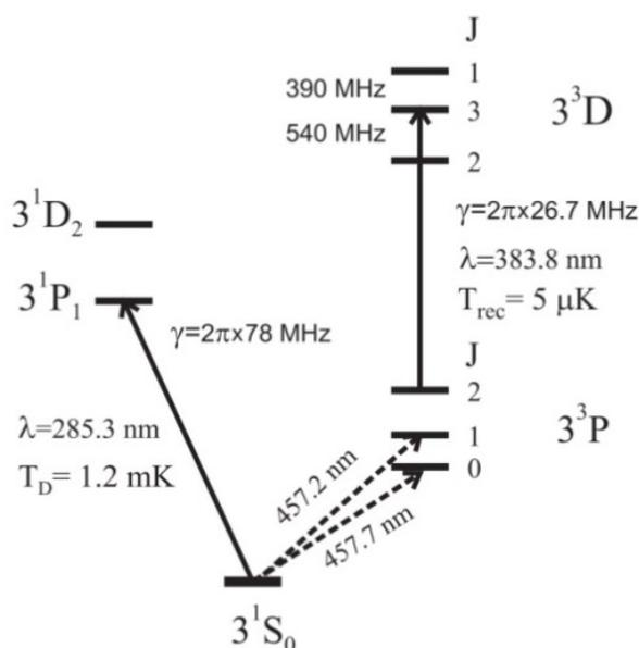
**Figure 1.** Simplified term diagram of  $^{24}\text{Mg}$  atoms. Solid lines denote the cooling transitions with corresponding temperature limits, while dashed lines denote possible “clock” transitions, which can be used for laser frequency stabilization.
