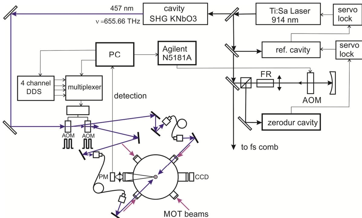
**Figure 2.** Simplified schematic of the experimental setup, showing the 914 nm Ti:Sa laser, the cavity with  $\text{KNbO}_3$  crystal for frequency doubling to the “clock” wavelength of 457 nm, the reference cavity for Ti:Sa laser linewidth preliminary narrowing, the zerodur cavity with a two pass acousto-optical modulator (AOM) for frequency stabilization and fine tuning of the clock laser frequency, the MOT with a detection system.
