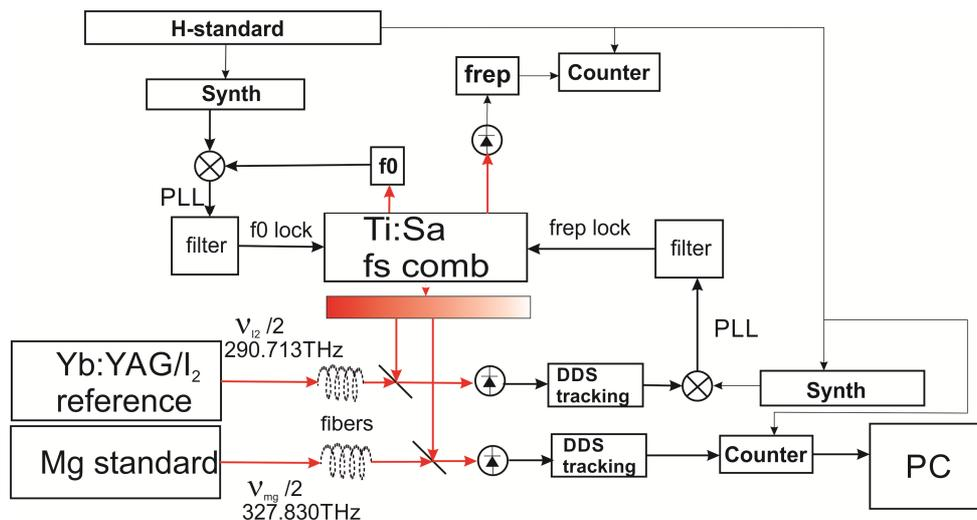
**Figure 4.** Scheme of the experimental setup for a frequency stability measurement of the clock laser system.
