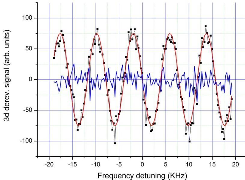
**Figure 3.** The error signal (a third harmonic of Ramsey fringes) that used for frequency stabilization (black line and symbols), red line is a sinusoidal fit of the error signal, blue line is a difference between the error signal and the fit. Blue line characterizes a signal/noise ratio  $S/N=6$ , an averaging time is  $\tau = 0.2 \text{ s}$  for a point (total curve comprises 144 points).
