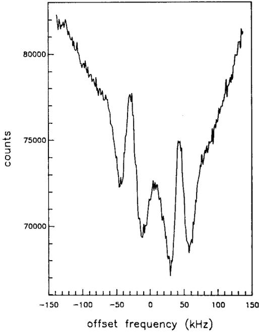
**Fig. 2.** Scan of the central part of the  $^{24}\text{Mg}$  intercombination line, showing the Lamb dip with superimposed Ramsey fringes
