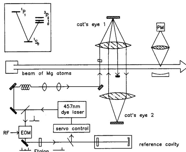
**Fig. 1.** Experimental setup and relevant part of the atomic level scheme
