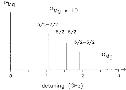
**Fig. 3.** Overview of the Mg intercombination transition with hyperfine and isotope structure. The amplitudes correspond to the observed intensities ( $^{25}\text{Mg}$  components multiplied by 10)
