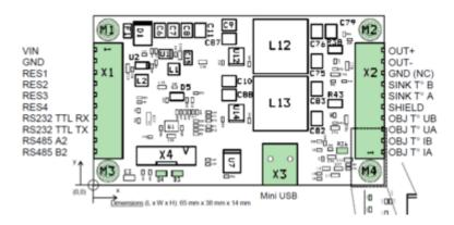
Different connectors were used for X1 and X2: PSK for X1 JAE for X2
