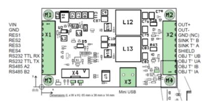
Different connectors were used for X1 and X2: PSK for X1 JAE for X2
