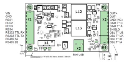
Different connectors were used for X1 and X2: PSK for X1 JAE for X2 Last update: 2018/05/08 groups:mg:temperature\_controller https://iqwiki.iqo.uni-hannover.de/doku.php?id=groups:mg:temperature\_controller&rev=1525769441 08:50
