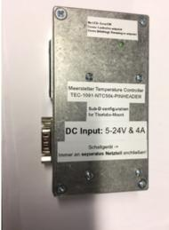
• The subD9 connector is used to connect the Meerstetter to the Thorlabs mount for the laser
