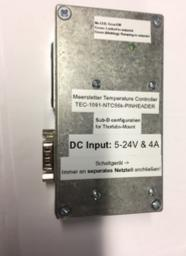
• The **subD9 connector** is used to connect the Meerstetter to the Thorlabs mount for the laser diode and is configured specially for that purpose.
