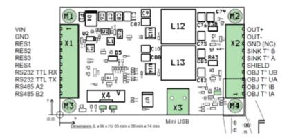
Different connectors were used for X1 and X2: PSK for X1 JAE for X2
