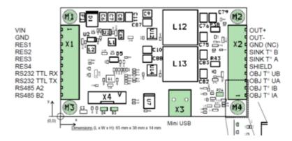
Different connectors were used for X1 and X2: PSK for X1 |AE for X2
