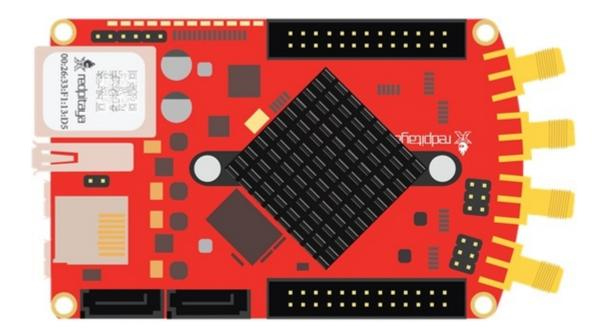
The FPGA-Board has 4 fast analog inputs and outputs. You can define them as whatever you want, but only the SMA connectors which are marked as 'In1' and 'In2' possess jumpers which allow you to choose between a Low Voltage Range (LV, +-1V) and a High Voltage Range (HV, +-20V). The board provides several more connectors depending on which board you have.
