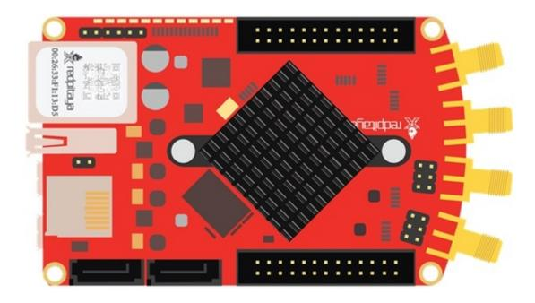
The FPGA-Board has 4 fast analog inputs and outputs. You can define them as whatever you want, but only the SMA connectors which are marked as 'In1' and 'In2' possess jumpers which allow you to choose between a Low Voltage Range (LV, +-1V) and a High Voltage Range (HV, +-20V). The board provides several more connectors depending on which board you have.
