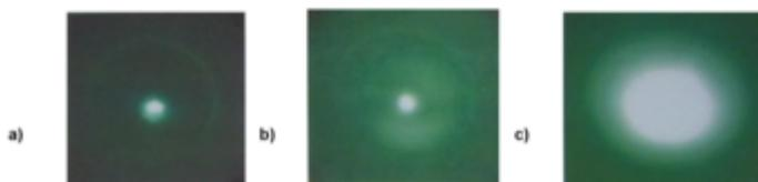
Figure 20: a) IR image of the cladding mode, a bright sharp dot inside a ring. b) IR image of the out coupling mode, core and cladding mode are mixed. c) IR image of the core mode.
