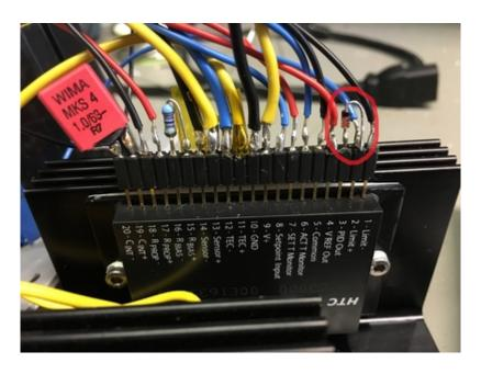
The direction of this diode is determined by whether you are using an NTC or a PTC sensor.
