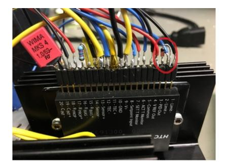
The direction of this diode is determined by whether you are using an NTC or a PTC sensor.
