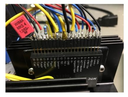
If it is plugged in correctly, the two wires coming from the back panel should connect to pin 9 "V+" and pin 10 "GND" of the HTC.
