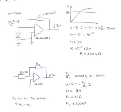
The optical amplifiers are limited by non-linear behavior above a voltage of 3V
