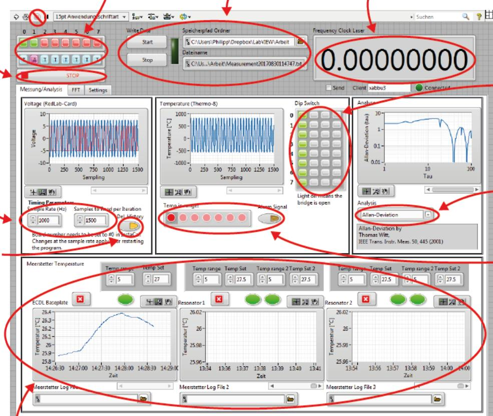
The timing parameters define how many samples to read within the time given with the sample rate until the graph can be shown.
