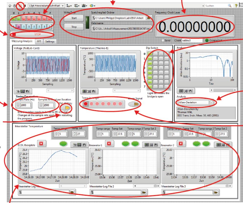
The timing parameters define how many samples to read within the time given with the sample rate until the graph can be shown.
