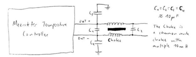
The capacitors used were the big red foil capacitors by Wima with a capacitance of ca.  $10\mu F$ . The choke is a  $\bigcirc$  common mode choke with multiple tens of mH.
