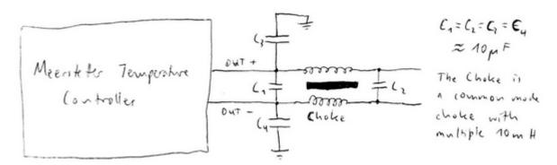
The capacitors used were the big red foil capacitors by Wima with a capacitance of ca.  $10\mu F$ . The choke is a  $\bigcirc$  common mode choke with multiple tens of mH.
