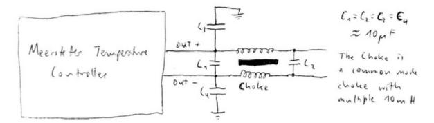
The capacitors used were the big red foil capacitors by Wima with a capacitance of ca. 10µF. The choke is a **p** common mode choke with multiple tens of mH.
