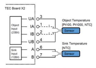
\* In case of Pt100 or Pt1000, use 4 wires to connect the Object Temperature Sensor
