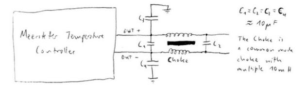
The capacitors used were the big red foil capacitors by Wima with a capacitance of ca.  $10\mu$ F. The choke is a  $\square$  common mode choke with multiple tens of mH.
