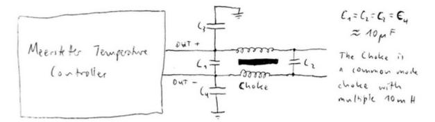
The capacitors used were the big red foil capacitors by Wima with a capacitance of ca.  $10\mu$ F. The choke is a  $\square$  common mode choke
