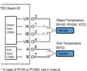
\* In case of Pt100 or Pt1000, use 4 wires to connect the Object Temperature Sensor
