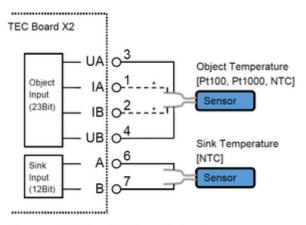
\* In case of Pt100 or Pt1000, use 4 wires to connect the Object Temperature Sensor
