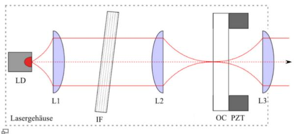
ECDL from top-view. LD: Laserdiode, Lx: Lenses, IF: Interference Filter, OC: Outcuppling Mirror, PZT: Piezo
