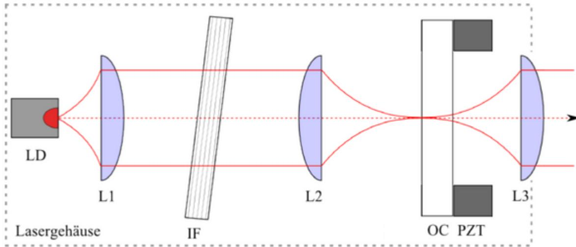
ECDL from top-view. LD: Laserdiode, Lx: Lenses, IF: Interference Filter, OC: Outcoupling Mirror, PZT: Piezo
