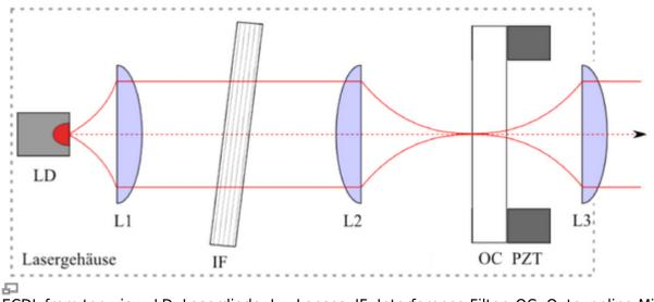
ECDL from top-view. LD: Laserdiode, Lx: Lenses, IF: Interference Filter, OC: Outcuppling Mirror, PZT: Piezo
