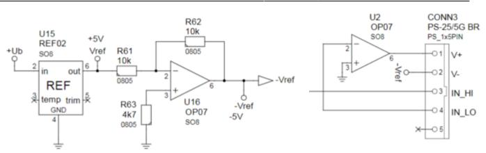
The Vin+ input (In High) is directly connected to the HTC T-Monitor Outputs.
