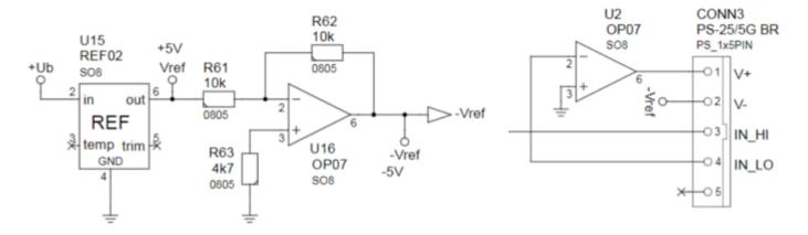
The Vin+ input (In High) is directly connected to the HTC T-Monitor Outputs.
