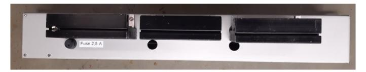
Here you find a 2,5 A fuse, protecting the circuitry and the heatsinks for the controllers.
