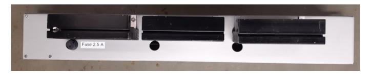
Here you find a 2,5 A fuse, protecting the circuitry and the heatsinks for the controllers.
