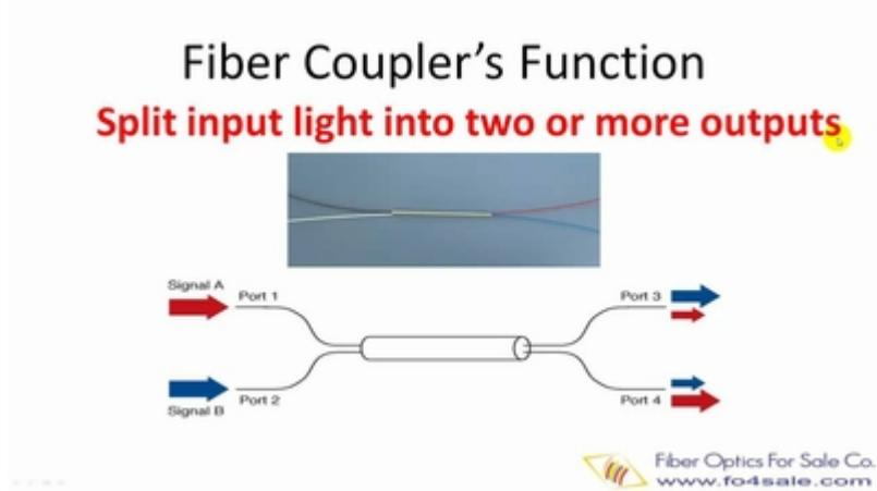
How Are Fused Fiber Optic Couplers Made & How Do They Work:
