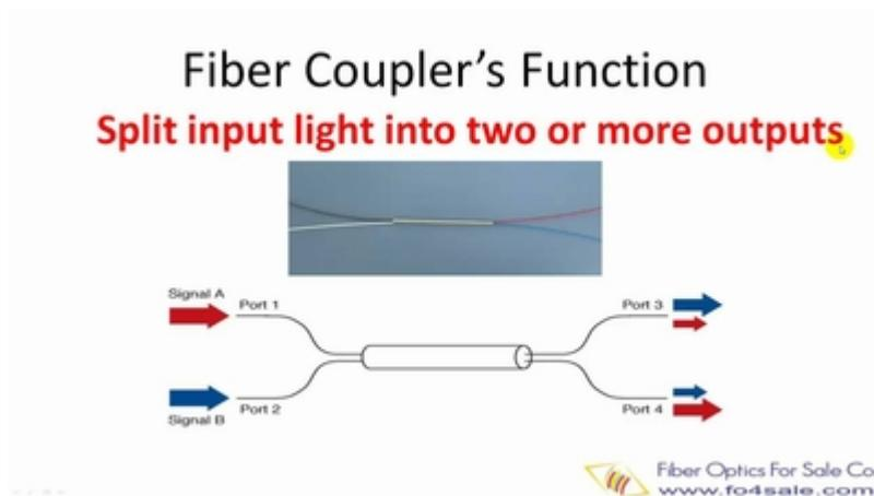
How Are Fused Fiber Optic Couplers Made & How Do They Work:
